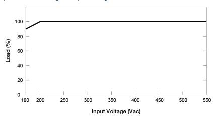
No output power de-rating for the input voltage range from 200 Vac to 550 Vac
