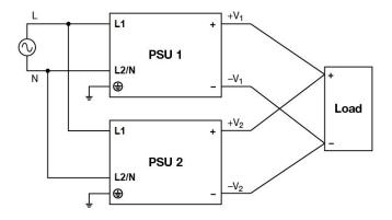
Fig. 5 Parallel Operation Connection Diagram
