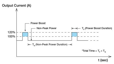
Fig. 3 Duty Cycle Calculation
