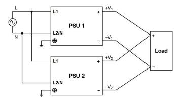
Fig. 5 Parallel Operation Connection Diagram
