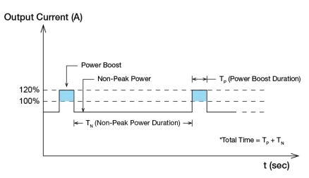
Fig. 3 Duty Cycle Calculation
