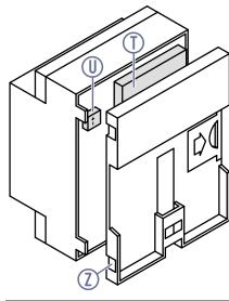
The typical estimated life of the battery is about 2 / 3 years and will gradually lose the capacity to hold a charge.
