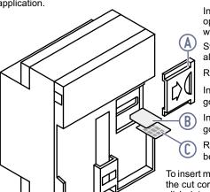
Install SIM card before to operate units equipped with PLMN module.
