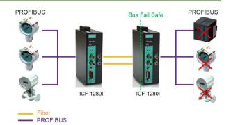
automatically detect the baudrate of the PROFIBUS device and apply this baudrate directly. This is an extremely convenient feature. If necessary, baudrates can be set to a fixed value via DIP switches to shorten the baudrate detection period when the system initializes.
