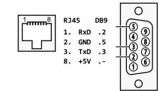
EIA-RS-232 (DCE) 115200 bit/s 8 DATA NO PARITY 1 STOP
